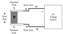
In the thermoelectric industry, 'P-type' semiconductor pellets are also employed. P-type pellets are manufactured so that the charge carriers in the material are positive (known in electronics
