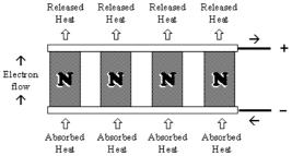
The only realistic solution is to wire the semiconductors in series, and doing so in a way that keeps them thermally in parallel (i.e., pumping together in the same direction). Here, we might
